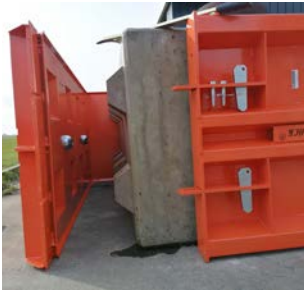
When the mold is opened, the magnet remains in the mold
