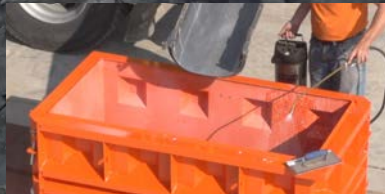
Applying oil into the mold
