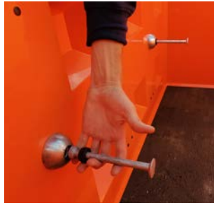
Place the rubber (BBGRO02) around the anchor (BBHA025)
