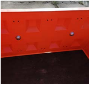
Place the magnet (BBMAG01) in the middle center of the mold
