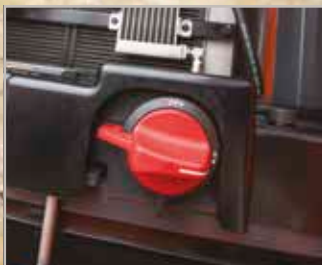
Battery cut-off switch
